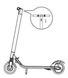
1. Remove the electric scooter from its box and unfold it. Lock riser in upright position. Plug handlebar wire loom into riser wire loom.
