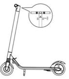
Attach handlebar to riser using 4 enclosed screws as per diagram.
